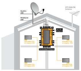
The following diagram illustrates a typical MDU/building installation with two Wideband LNBs receiving two satellites:
