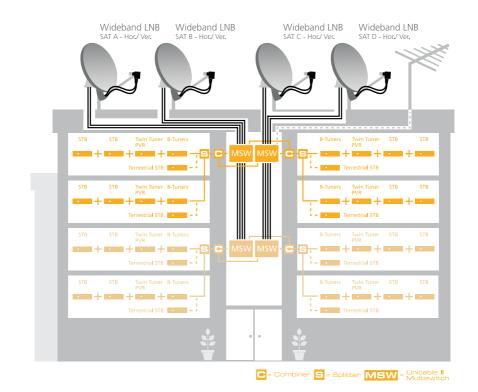
Connect the cables from the Wideband LNBs to the input connectors marked with Sat A/C Vertical and Horizontal and Sat B/D Vertical and Horizontal (pay attention to identification of the Wideband LNB connectors).
