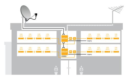
Connect the cables from the Quattro LNB to the input connectors marked with LNB V/L, V/H, H/L and H/H inputs (pay attention to identification of the Quattro LNB connectors). The multiswitch is equipped with Terrestrial input. Connect the Terrestrial antenna to this input:
