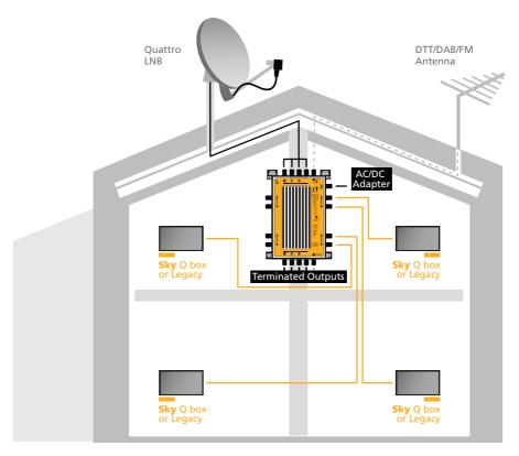
The following diagram illustrates a typical MDU/building installation:
