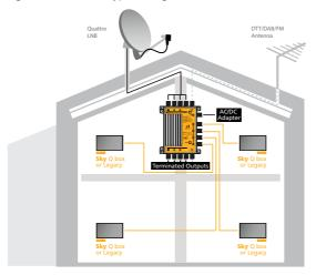
The following diagram illustrate a typical MDU/building installation:
