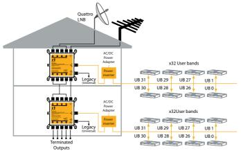
Connect the cables from the Quattro LNB to the input connectors marked with LNB V/L, V/H, H/L and H/H inputs (pay attention to identification of the Quattro LNB connectors). The multiswitch is equipped with Terrestrial input. Connect the Terrestrial antenna to this input:
