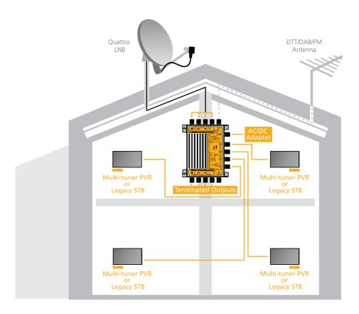
Connect the cables from the Quattro LNB to the input connectors marked with LNB V/L, V/H, H/ Land H/H inputs (pay attention to identification of the Quattro LNB connectors). The multiswitch is equipped with Terrestrial input. Connect the Terrestrial antenna to the Terrestrial input port.
