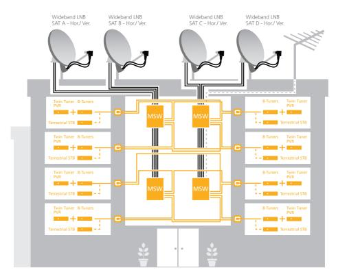
Note: The four satellite installation requires the output ports of the two Multiswitch units to be connected to an external combiner as shown in the diagram (to provide for DiSEqC 2.0 communication, the combiner should support bidirectional pass through for DC and 22kHz signals).
