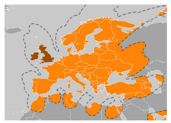
KA-SAT is the first High Throughput Satellite (HTS) in Europe and marks a new generation of multi-spotbeam high-capacity satellites. It is positioned at 9° East and covers Europe and the Mediterranean basin and has 82 tight Ka-band spot beams across Europe. Source: Eutelsat
